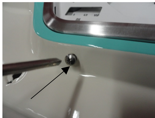
Picture showing bottom left mounting bolt
