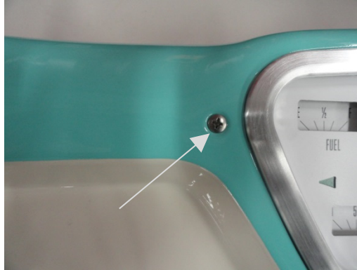
Picture showing left front mounting bolt
