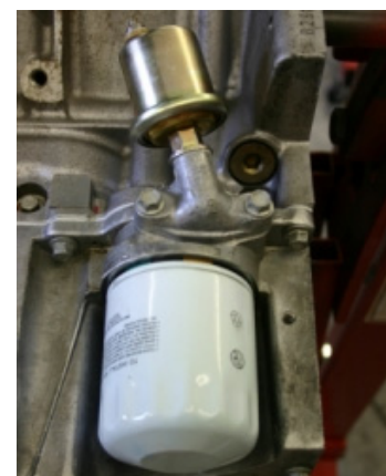
LS1 Oil Bypass Housing
