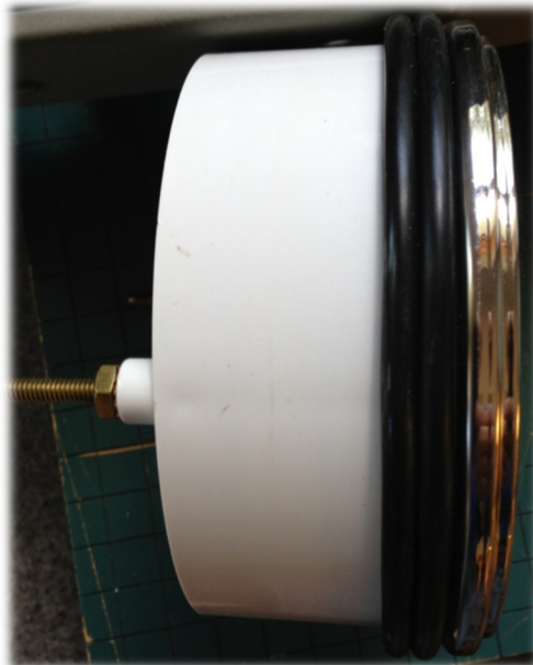
Two O-rings installed on a gauge
