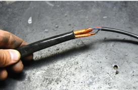
The oil pressure sensor comes with a three-wire pigtail so you need to connect a power, signal, and ground wire. This sensor also operates with 5 volts rather than resistance, which allows for a compact sensor. We added a heat sleeve to protect the wires and routed the sensor ground back to the same point as the other gauges.
