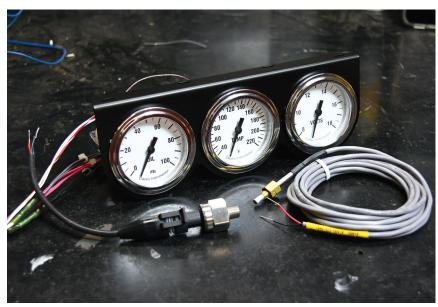
With the main wires connected, it was time to install the panel under the dash then get to work on the temp and pressure sensors.
