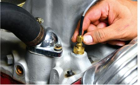
The low-temp gauge (40 to 220 degrees) uses a 5-volt sensor rather than a usual resistance-based sensor. The voltage signal is much more accurate for the fullsweep gauge. Classic has found it best to install the sensor in the intake manifold but the cylinder head is acceptable when a port is not available such as on LS intakes).
