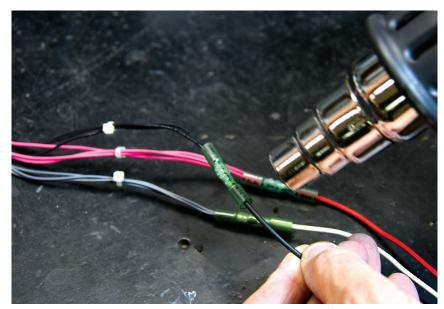
Each gauge requires switched 12 volts, ground and a wire for the lights. We put each of the wire groupings into one heat-shrink butt connector and ran a single wire to its connection on the car.
