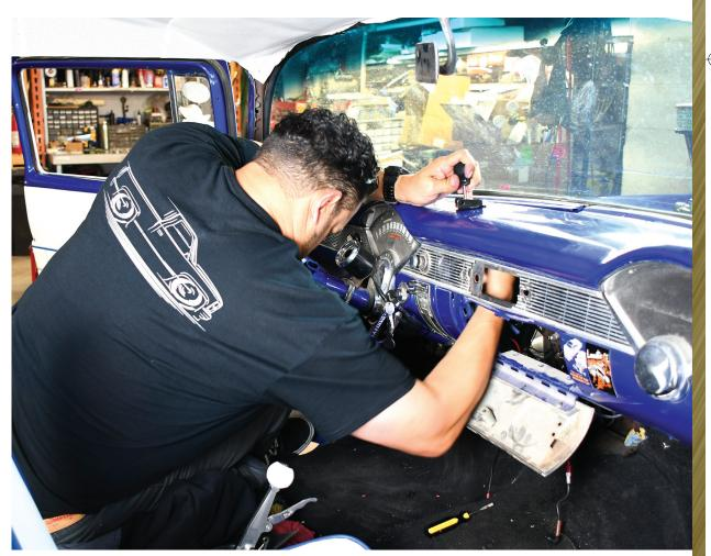
Several yoga positions were needed to reach up under the dash to mount the tach and finish off the wiring.
