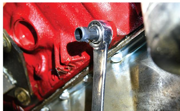
Thanks to the fenderwell headers, there was plenty of room to mount the oil-pressure sensor on the side of the block.
