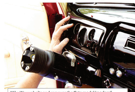
Mike Way unbolts and removes the "late model/modern" gauges and panel from his dad's dashboard.
