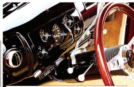
This is typical of what many rodders would do to update the original gauges to 12 volt and also to customize their street rod.
