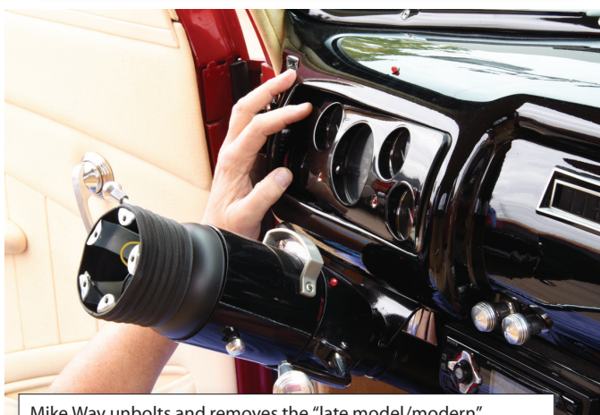
Mike Way unbolts and removes the "late model/modern" gauges and panel from his dad's dashboard.
