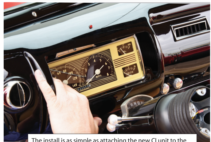
The install is as simple as attaching the new CI unit to the stock studs and running the wire to the included senders.
