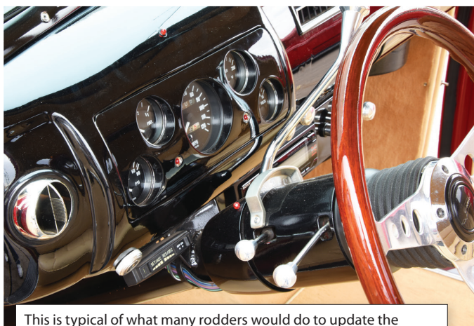
This is typical of what many rodders would do to update the original gauges to 12 volt and also to customize their street rod.
